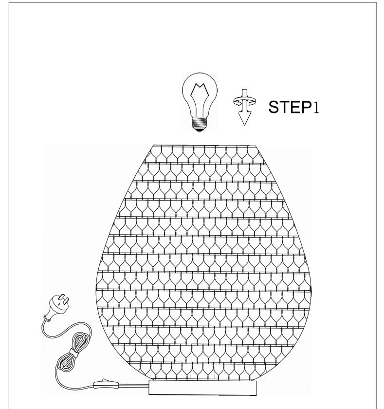
THIS ITEM HAS A "TYPE Y" CORD IF THE EXTERNAL FLEXIBLE CABLE OR CORD OF THIS LUMINAIRE IS DAMAGED, IT SHALL BE EXCLUSIVELY REPLACED BY THE MANUFACTURER OR HIS SERVICE AGENT OR A SIMILAR QUALIFIED PERSON IN ORDER TO AVOID A HAZARD.
