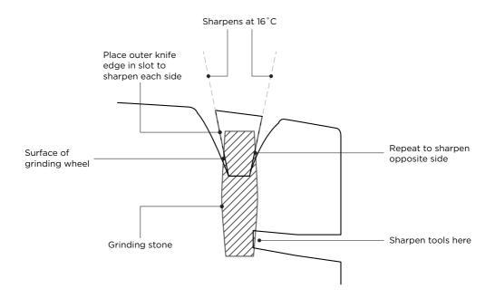
the length of the blade and do not interrupt or stop the motion when in contact with grinding wheels.
