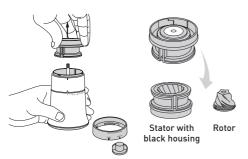
4. Unscrew the nut anti-clockwise from the end of the shaft and then pull the ceramic grinding unit out of the hopper. The ceramic grinding unit includes a rotor and a stator. Rinse parts under running water. Dry thoroughly before replacing parts and storing. Tip: a kitchen brush is handy for cleaning under tap.
