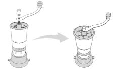
Unscrew the nut and take out the white washer from threaded shaft. Attach the crank to the threaded shaft, making sure that the hexagonal shape on the crank fits into the hexagonal hole at the end of the threaded shaft.
