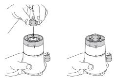
4. Place the nut back onto the shaft and turn it clockwise until screwed tight. Tip: Hold the crank still and screw the nut a little closer to rotor with white support. This will help the finest grind setting grind even finer
