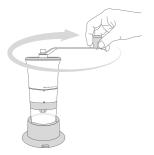
2. Once the rubber suction base is attached firmly to the countertop and beans are within the hopper, grab the knob of crank and turn clockwise.
