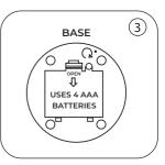
Insert the DC plug into the back of the Plasma Ball base. Plug the USB cable into a power source.  For battery use ensure the device is unplugged and the switch is on the OFF position. Insert 4x AAA batteries (not included).
