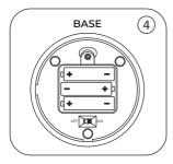
4. For battery use unscrew and remove the battery cover. Insert 3 x AA batteries (not supplied) with the correct polarity, then replace the battery cover and screw back into place. If using USB please ensure batteries are removed. The Mist Lamp has an in-built power saving mode. When switched on, the motor will run for 5 seconds and pause for 5 seconds.
