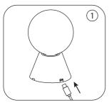
Insert the USB-C plug into the back of the Mist Lamp base
